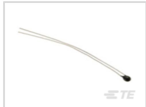
Discrete NTC Sensor Type: **Epoxy Coated NTC Thermistor**Wire Connection: **Open End**Discrete NTC Wire Length: **76 mm**Resistance (at 25°C): **1 kΩ**β-Value(25/85): **3348 K****Features****Product Type Features**
